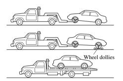
When towing with the rear wheels on the ground, release the parking brake.
