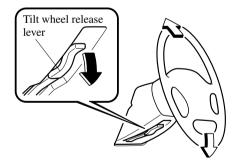
After adjusting, push the wheel up and down to be certain it's locked before driving.
