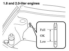
Pull it out again and examine the level. It's OK between L and F. But if it's near at or below L, add enough oil to bring the level to F.
