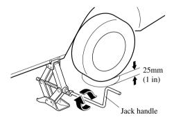
6. Remove the lug nuts by turning them counterclockwise; then remove the wheel.
