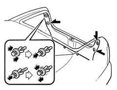
2. Remove the inside cover's plastic retainers and partially open the inside cover.
