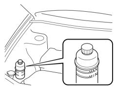
The level must be kept between MIN and MAX.
