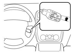
Your vehicle has a tap-up feature that allows you to increase your current speed in increments of 1.6 km/h (1 mph) by a momentary tap of the lever. Multiple taps will increase your vehicle speed 1.6 km/h (1 mph) for each tap.
