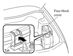
3. If a fuse is blown, replace it with a new one **of the same rating.**
