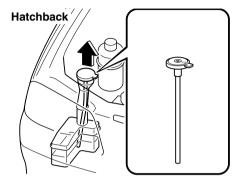
To inspect the washer fluid level in the front reservoir, pull off the cap. Then, holding your thumb over the hole in the center of the cap, lift it straight up. There should be fluid in the straw. Add fluid if necessary.
