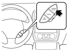
Your vehicle has a tap-up feature that allows you to increase your current speed in increments of 1.6 km/h (1 mph) by a momentary tap of the RESUME/ACCEL button. Multiple taps will increase your vehicle speed 1.6 km/h (1 mph) for each tap. • (Type A)
