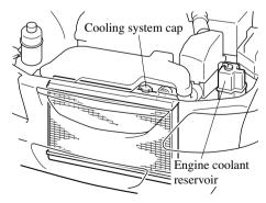
If you find no problems, the engine is cool, and no leaks are obvious, carefully add coolant as required (page 8-14).
