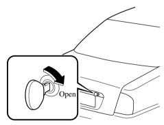
To close, use both hands to push the lid down until the lock snaps shut. Don't slam it.
