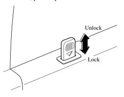
To lock any door with the door-lock button from the outside, push down its door-lock button and close the door.
