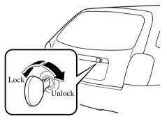
To unlock the liftgate with the key, insert the key and turn it clockwise.
