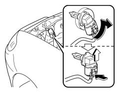
12.Install the new bulb in the reverse order of removal.
