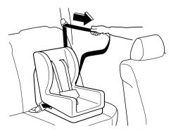
3. Push the child-restraint system firmly into the vehicle seat. Be sure the belt retracts as snugly as possible. Clicking from the retractor will be heard during retraction if the system is in the automatic locking mode. If the belt does not lock the seat down tight, repeat this step.
