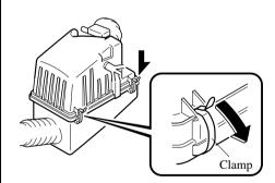
2. Lift off the air filter cover and remove the filter.
