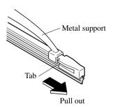
3. Remove the metal stiffeners from the blade rubber and install them in new blades.
