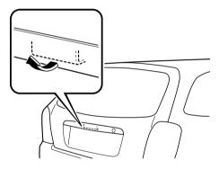
To close, use both hands to push the liftgate down until the lock snaps shut. Do not slam it. Pull up on the liftgate to make sure it is secure.
