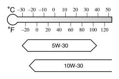
When choosing an oil, consider the temperature range your vehicle will operate in before the next oil change. Then select the recommended viscosity from this chart.
