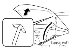
Before closing the hood, secure the rod in its clip.
