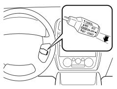
Your vehicle has a tap-down feature that allows you to decrease your current speed in decrements of 1.6 km/h (1 mph) by a momentary tap of the lever. Multiple taps will decrease your vehicle speed 1.6 km/h (1 mph) for each tap.
